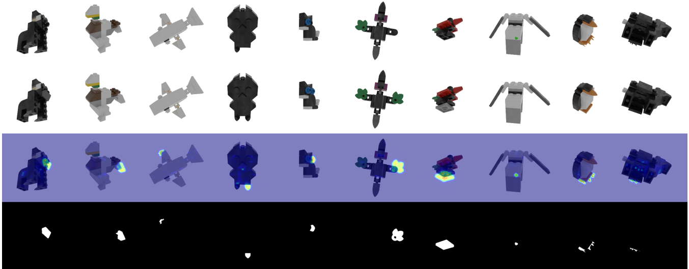
Figure 1: Visualization of the Pose-agnostic Anomaly Detection result. From top to bottom: the test image, the rendered image, the heat-map of predicted anomaly score map, and the ground truth.
